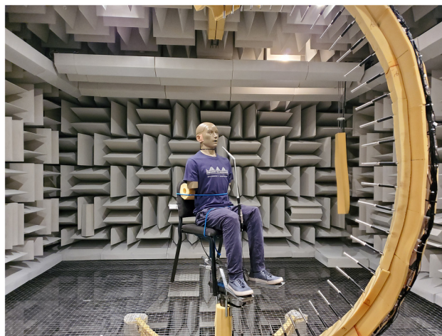
FIG. 10. (Color online) KEMAR HATS seated within a directivity measurement system.
