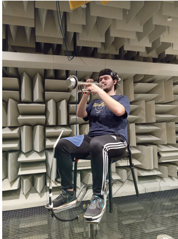
Figure 2: Seated musician with the head restraint, clip-on tuner, and trumpet-mounted laser before the straight-mute measurements.
