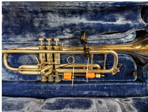
Figure 3: Bach Stradivarius Model 43 B♭ trumpet with a clip-on tuner and laser pointer attached.
