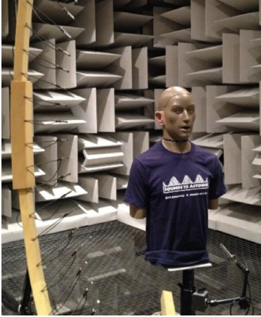
FIG. 3. (Color online) The GRAS KEMAR 45BC HATS positioned on a stand in the directivity measurement system. A fixed microphone attached to the stand rotated with the HATS to provide an alternative reference signal.
