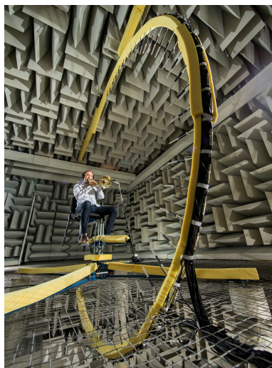
Figure 1: Microphone array used for measuring directivities of musical instruments and speech.
